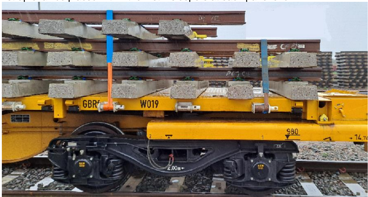
Example of securing strap positions with various length panel ends.
