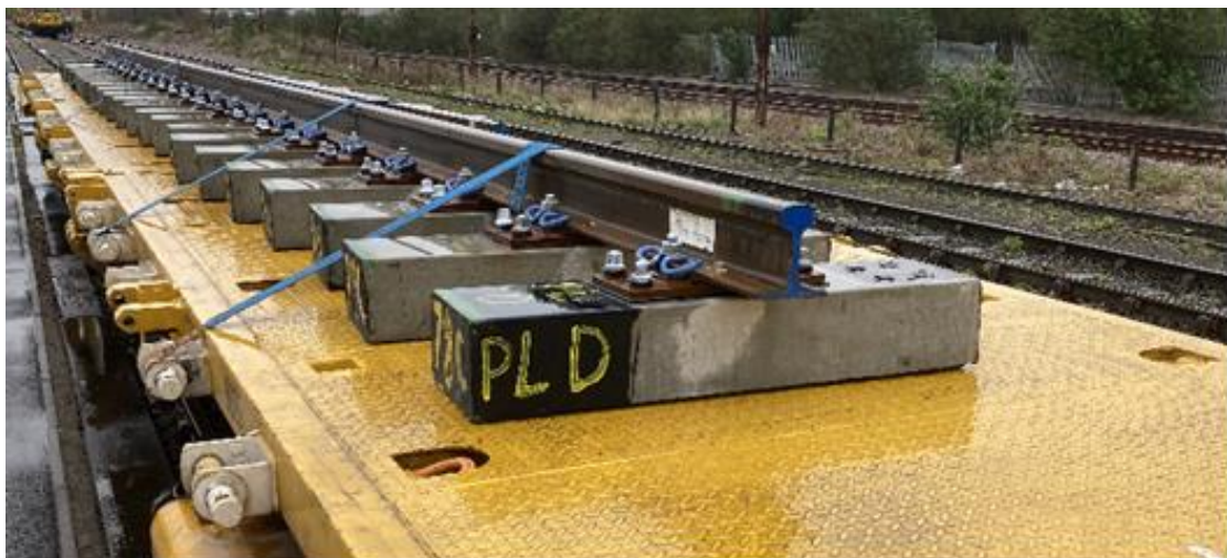
Stub panel loaded centrally.
